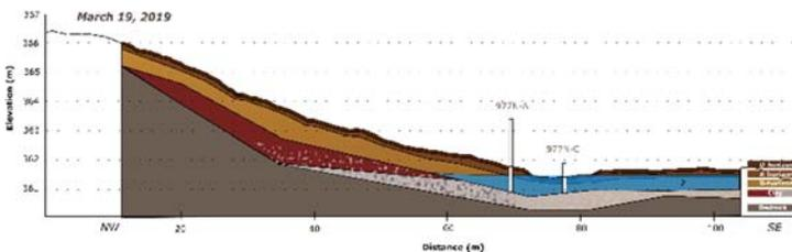
**Figure 3.** 977N wetland cross section. The water overlay shows aquifer on March 19, 2019 as determined from the water level readings from wells on the transect.
