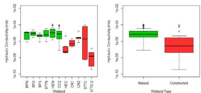
**Figure 1.** (A) Comparison of all K measurements for each wetland (B) Comparison of all K measurement for each wetland type.
