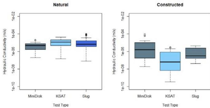
**Figure 2.** Comparison of test types' determination of K at natural (A) and constructed wetlands (B).
