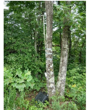
Fig. 2. Two microphone setup with SM3 acoustic monitor
